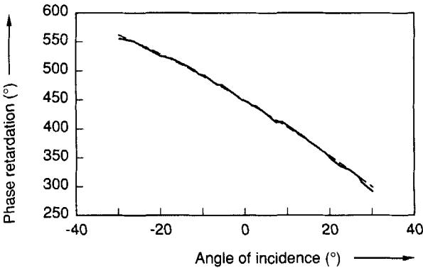
FIGURE 7 Phase retardation vs rotation angle for a 61.8 \mu\text{m} \text{SiO}_2 cell with \theta = 22.85^\circ . Measured at 25.0°C.
