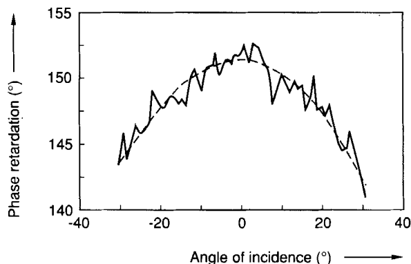
FIGURE 2 Phase Retardation versus rotation angle for a 1.91 \mu\text{m} thick PI cell with \theta = 0.27^\circ . Measured at 22.2^\circ\text{C} .
