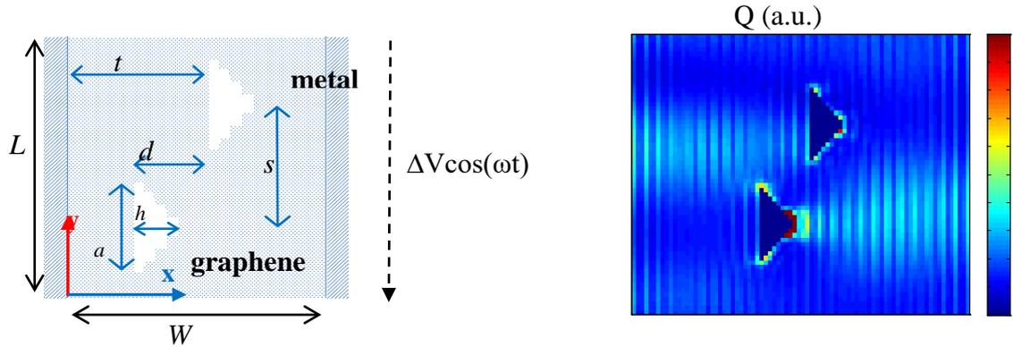
Figure 1. a) Triangular vacancy defect in paired configuration. (b) Top view of surface charge density  $Q$ . Here,  $\mu_c = 0.22$  eV, with  $d = 3$  nm,  $a = 7$  nm,  $h = 2$  nm,  $s = 9$  nm,  $t = 13$  nm.
